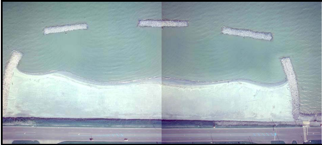
Figure 5. Aerial view showing increased accretion on west end of the beach taken on 11/24/2001 (Lanmon Aerial Photography, Inc.).
