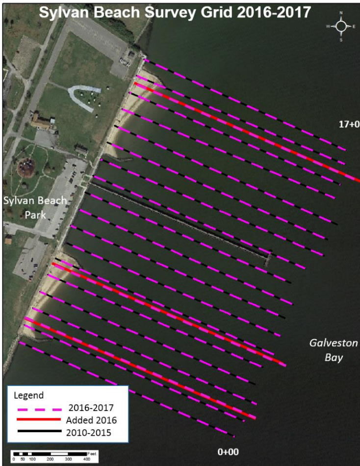
Figure 148. Transect location and orientation of the two beach cells at Sylvan Beach Park
