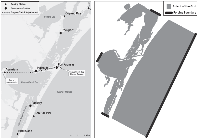
Figure 1(a). Study area map with locations of forcing stations and verification stations and (b) the model grid extent and location of water level forcing cells.
